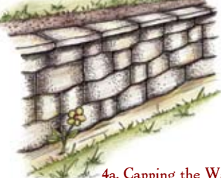
4a. Capping the Wall
